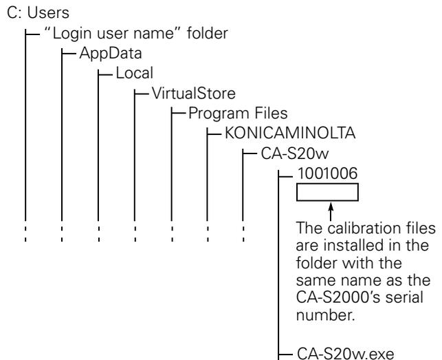
The calibration files are installed for each serial number (See page 9 “Status Bar” in the CA-S20w Instruction Manual.) of the CA-2000 to use.
